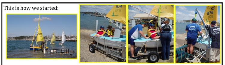
The only way to exchange sailors was to do so on-shore with the dinghy centre-boards and rudders raised and wheel-chair sailors lifted in and out via a crane mounted on the trailer frame. A volunteer then was located in the water to arrange the centre-boards/rudders as needed. This was a popular job during summer though not that attractive during winter.
